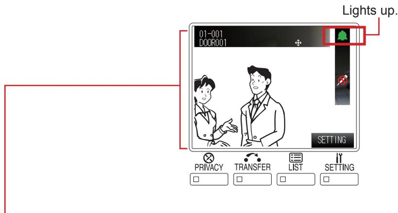
The station no., station name and video image at the calling station (following the symbol image) are displayed.
