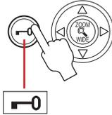
The door lock is released for the time set in the System setting on a PC.
