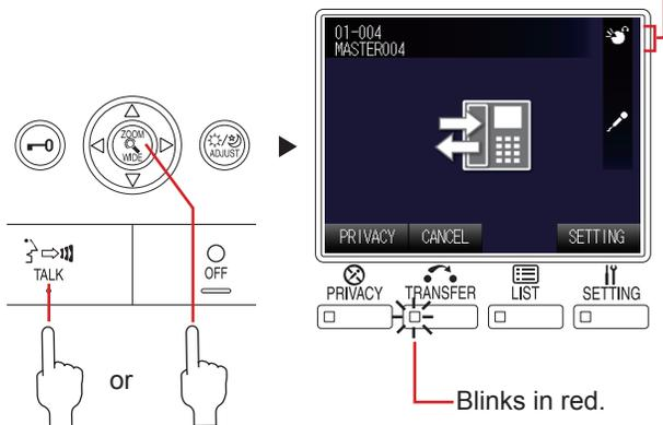
\* While transferring, a sound rings at the source station to indicate a transfer.
